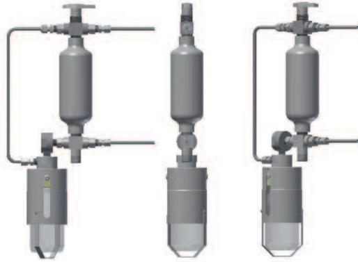
The ability to purge the sample point ensures optimal retrieval of a representative, contamination free sample. The S23 type sampler provides a system purge in addition to a fixed sample volume. No vent connection is needed. The vent is connected to the top valve. This way a loop is created in order to fill the bottle by means of gravity.
