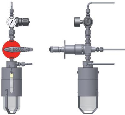
The ability to back purge the sample point ensures optimal retrieval of a representative and contamination free sample. The DPM type sampler in back purge configuration allows a gas to purge the sampler prior to sampling ensuring a fresh sample.
