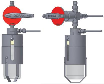
The ability to connect the sampler close to the sample point ensures optimal retrieval of a representative and contamination free sample. The DPM type sampler in on/off configuration allows the product to flow directly into the sampler via a two-way valve.
