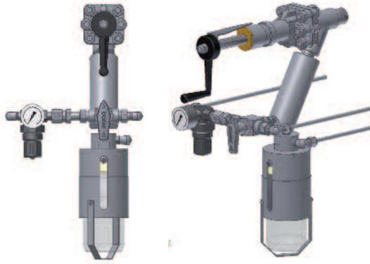
Being able to provide a jet purge adapter to a piston type sampling valve, ensures optimal retrieval of a representative, contamination free sample of high viscosity liquids. The DPJ type sampler allows purging of the sample valve outlet thus eliminating dead volume. In solvent purge configuration, the system allows for purging with a solvent or with nitrogen.
