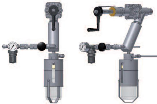
Being able to provide a jet purge adapter to a piston type sampling valve, ensures optimal retrieval of a representative, contamination free sample of high viscosity liquids. The DPJ type sampler allows purging of the sample valve outlet thus eliminating dead volume. The jet purge adapter has two flow paths. The first flow path allows the product to flow to the sample bottle and the second flow path enables the jet purge adapter to be purged with an inert gas.
