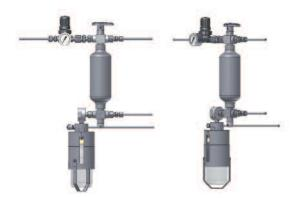
The ability to purge the sample point ensures optimal retrieval of a representative, contamination free sample. The S23 type sampler provides a system purge and needle purge in addition to a fixed sample volume.
